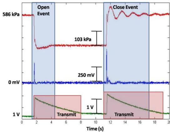
**Figure 2: A typical pressure wave showing the open and close events on a calibrated pressure sensor (red), and piezoelectric sensor (blue). Storage capacitor voltage during normal operation of the system (green)**
