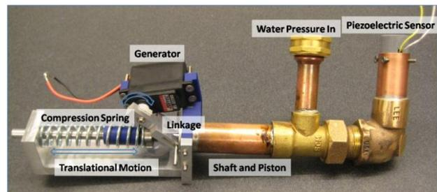
Figure 1: WATTR mechanical harvester and sensor
