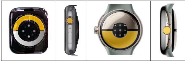
Figure 3: The ECG contact points (highlighted in yellow) for the Apple Watch Series 9 (two left images) and for the Google Pixel Watch 2 (two right images).
