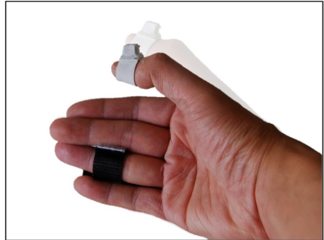
Figure 1. uTrack enables real-time 3D input from the thumb and fingers using one permanent magnet (thumb) and two magnetometers (ring finger).
