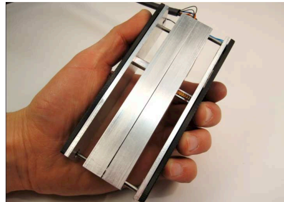
Figure 1: SqueezeBlock realizes virtual springs that can dynamically be altered to haptically convey information to a user.
