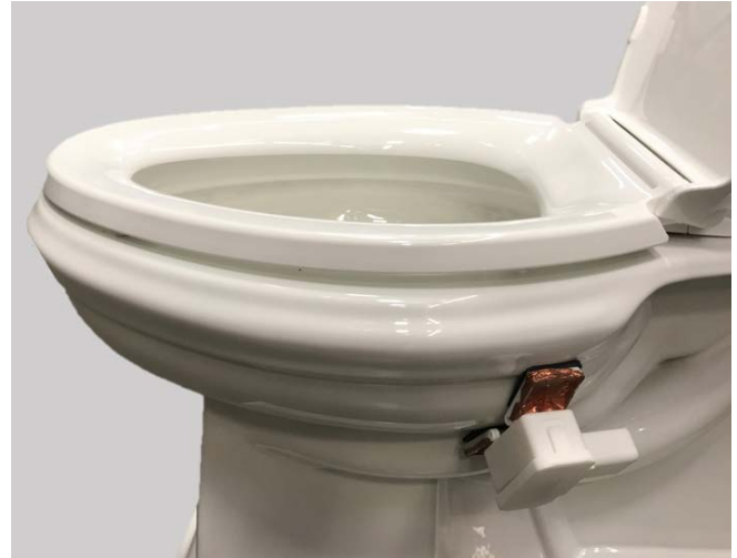
Figure 1. The RoyalFlush prototype, which has two adhesive copper plates that are attached onto the back of the toilet bowl.
