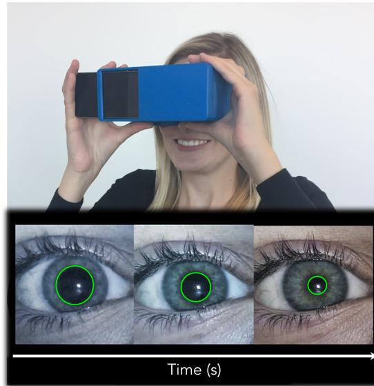
Fig. 1. PupilScreen is a system that measures the pupillary light reflex to determine the severity of a traumatic brain injury. A smartphone app records a video of the patient's eyes as the camera's flash illuminates them. The VR headset-like box controls the position of the phone and the lighting that reaches the eyes.
