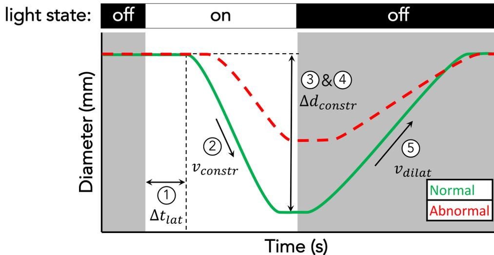
Fig. 2. A PLR curve annotated with the five common descriptive measures: (1) latency, (2) constriction velocity, (3) constriction amplitude, (4) constriction percentage, and (5) dilation velocity. An abnormal PLR curve with increased latency, slower velocities, and diminished amplitude is also included for comparison.
