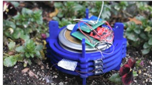
Figure 1. Temperature-based harvester and sensor node
