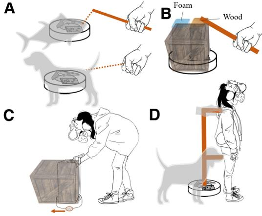
Figure 5. *MoveVR* can simulate a variety of force feedback with everyday objects as proxies. A: Tension using string/rope proxies between users and robots. B: Reaction with proxies built by different materials. C: Resistance by configuring the wheels' status. D: Impact from the robot crashing on users with varying speeds.
