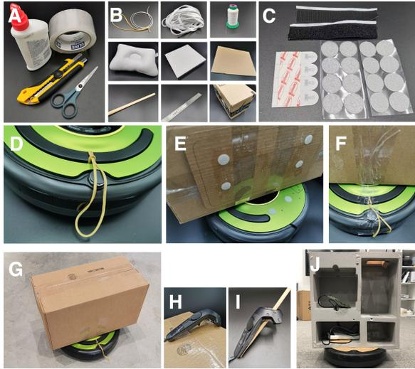
Figure 3. Fabricating and assembling MoveVR. A: Example of fabrication tools. B: Example of everyday objects as proxies. C: Touch fasteners or double-sided tape to fix the carry-on proxy. D: Attaching the shared-proxy onto the robot. E: Fixing the carry-on proxy using touch fasteners. F: Fixing the carry-on proxy using tapes. H - I: Attaching the VR controller with the user-driving proxy. G/J: Examples of MoveVR carrying proxies.
