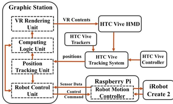
Figure 2. MoveVR system architecture.
