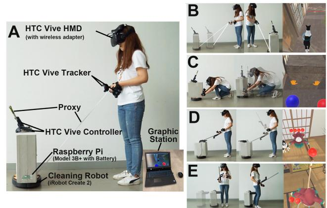
Figure 1. Overview of *MoveVR*. A: Hardware setup. B: Adjusting tension intensities and directions by configuring the relative position between the robot and the user. C: Multi-level resistance force feedback by configuring the robot's direction of motion. D: Simulating material rigidity through rotating different material proxies within reach of users. E: Applying different levels of impact force to users by varying the speed.
