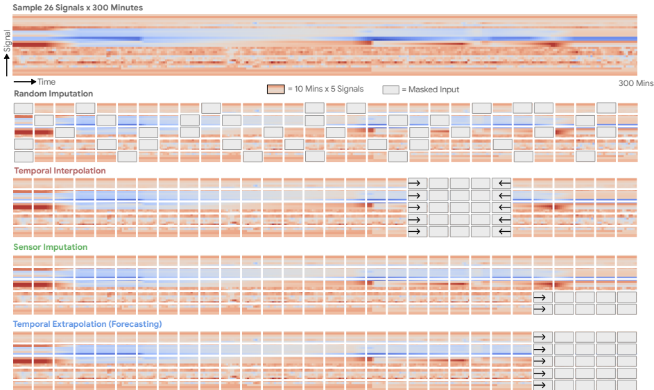
Figure 2: Generative LSM Tasks and Pretraining. We define four distinct generative tasks: random imputation, temporal interpolation, signal/sensor imputation, and temporal extrapolation (forecasting). Random imputation was empirically chosen as the pretraining task.
