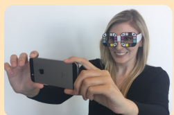
BiliScreen Smartphone-based system for assessing scleral jaundice
