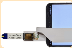
GlucoScreen A reimagined glucose strip that directly interfaces with a smartphone's touchscreen
