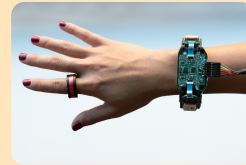
AuraRing Tracking accurate finger motion using magnetic sensing
