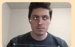
SlouchSense Using computer vision to assess sitting posture during computer use
