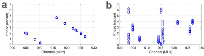
Fig. 5. Phase-channel relation (a) linear relation when still (b) non-linear under motion
