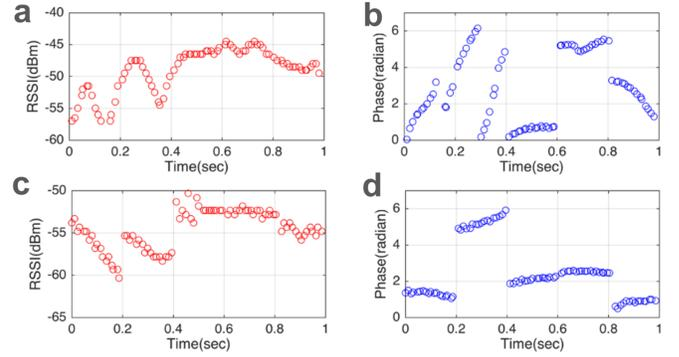
Fig. 4. Raw channel parameters of tag moving and interfered states. (a) RSSI-motion (b) phase-motion (c) RSSI-interference (d) phase-interference
