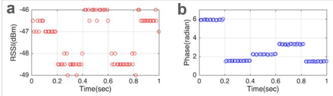
Fig. 3. Discontinuity in RSSI and phase samples due to carrier frequency sweep. (a): RSSI vs. time, (b): Phase vs. time
