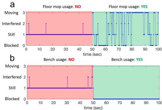
Fig. 9. Correlation between tag states and object usage: (a) example mobile object: floor mop, (b) example static object: sitting bench
