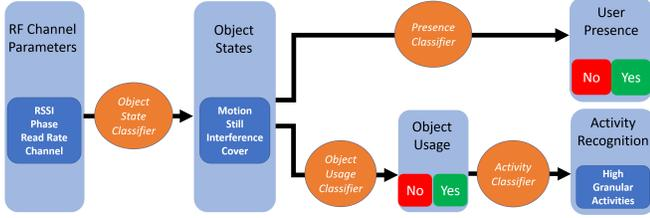
Fig. 2. An overview of our activity recognition pipeline: from RF channel parameters to sensing object usage, detecting user presence and recognizing daily activities.
