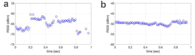
Fig. 6. RSSI variations of 2 tags attached to two objects of different materials at 2 different locations
