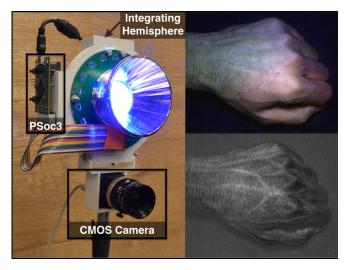
**Figure 1.** (*Left*) HyperCam Hardware. (*Top-Right*) RGB image of a user's hand. (*Bottom-Right*) The user's veins and skin texture are emphasized in the HyperCam-generated image.
