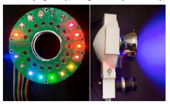
**Figure 4.** (*Left*) 17 LEDs of different wavelengths form HyperCam's spectra. (*Right*) The LEDs shine inside the integrating sphere (white enclosure) and the light comes out of the opening in the center.
