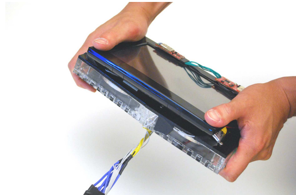
Figure 1: GyroTab provides reactive torque feedback. Two masses (under the display) spinning in opposite directions are controlled to produce varying levels of feedback that oppose the user's movement.
