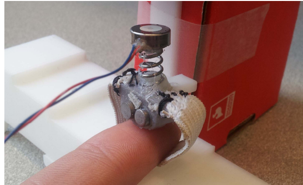
Figure 1. The prototype impedance adapter in test setup for displacement measurement.
