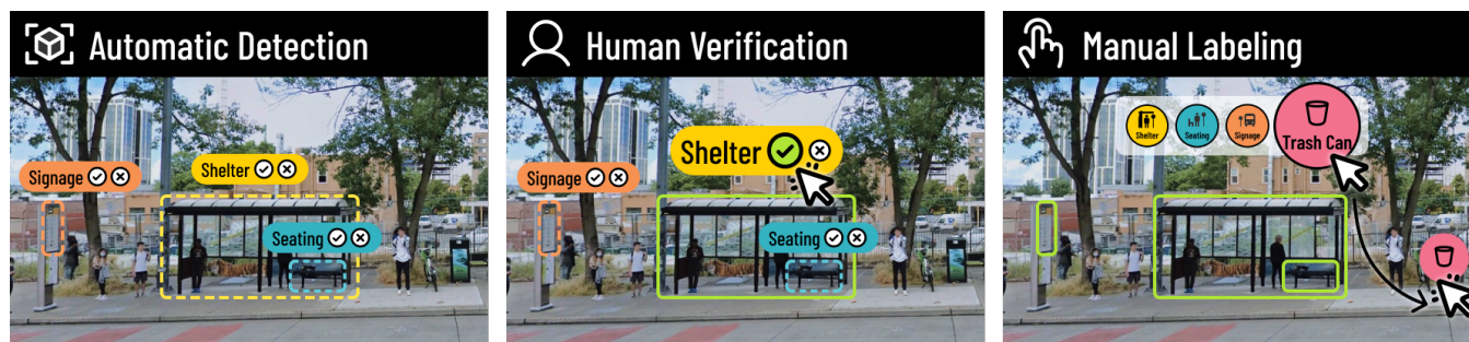
Figure 1: The BusStopCV human+AI data collection workflow: a real-time YOLOv8 CV model automatically detects bus stop features such as shelters and benches in streetscape imagery (left). Users can verify detections via lightweight click interactions (middle) or manually label features not detected by the model (right). Verified bounding boxes turn from dashed to solid lines. See demonstration video in supplementary materials.
