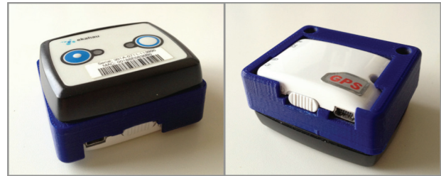
Figure 1. A single sensing tag of uLocate with dimension of 54x45x26 (mm). (Left) WiFi tag for the indoor tracking. (Right) GPS logger with a customized cap for the outdoor tracking.
