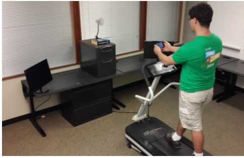
Figure 7. To support the different conditions, the experimental setup included a treadmill for walking, a lamp for consistent lighting, and a monitor on either side for distractions.
