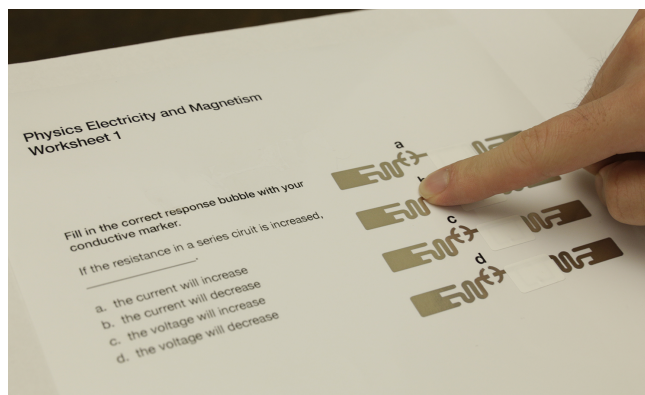
Figure 7. In this polling application, a student can pick a response on a worksheet and receive live feedback.
