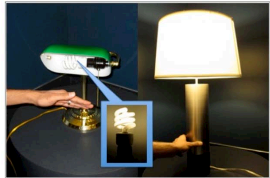
Figure 1: A user performing a hover gesture (left) near a compact fluorescent light (CFL) lamp, and a user touching the metallic base of a lamp (right). Both of these gestures can be detected using a single plug-in module.
