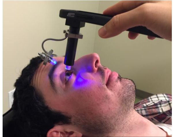
Figure 1. The proposed system emulates fixed-force applanation tonometry using the hardware adapter pictured above. The clear acrylic cylinder is allowed to move freely within the black casing so that its mass provides a constant force on the patient’s eye.
