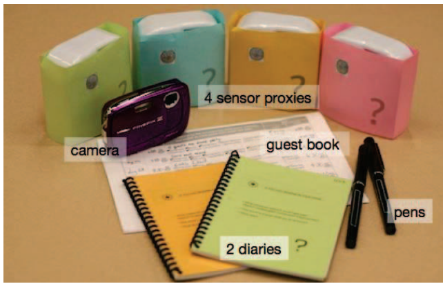
Figure 4. The take-home study package contained 4 sensor proxies (off-the-shelf motion sensor lights wrapped in decorative paper), 1 digital camera, 2 diaries, and 1 guestbook.
