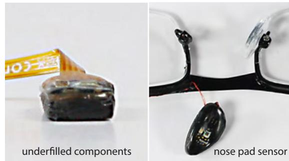
Fig. 7. To limit the exposure of our sensor boards to the user’s skin and protect them from external influences, such as sweat, we *underfilled* all components using fine traces of hot glue that we manually reflowed. Using an underfill keeps the main components of the sensor board exposed to make direct contact with the wearer’s skin, such that the LED and the photodiode optimally inject light into the skin and observe optimal reflections, respectively.
