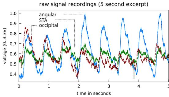
Fig. 9. Raw signal captured by the sensors, here a particularly bad example due to the opamp recovery from railing intensities just before restoring the proper amount of signal amplification.
