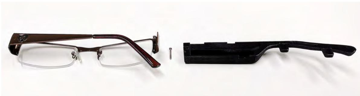
Fig. 8. Mechanical design of the frame. The ABS-printed frame is parametric for easy adjustment to each wearer’s head dimensions. Cavities accommodate the main board and the sensor boards. The groove along the frame routes FPC cables between all boards. We close the frame using black tape.
