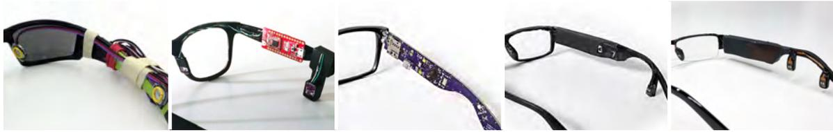
Fig. 3. The iterative evolution of our Glabella prototypes. While the first two prototypes consisted of Arduino-based components to study and evaluate the feasibility of our approach in pilots, Versions 3–5 miniaturize the form factor into an integrated device that comprises all components on two separate types of boards: the main board, which sits inside the glasses frame, and the sensor boards that connect through flex PCB cables.
