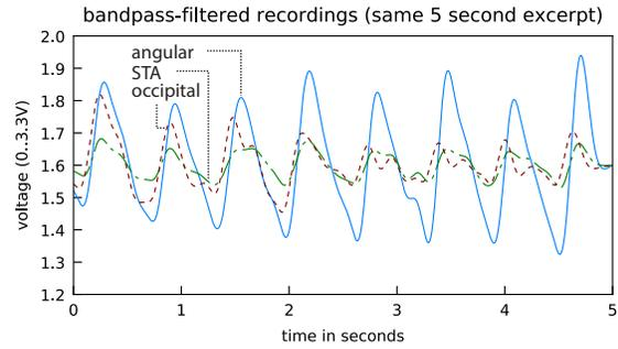
Fig. 10. After applying a 0.4 Hz–8 Hz bandpass filter to the raw intensities, the pulse reflections exhibit clearly their characteristic features, which we consequently detect for extracting timestamps.
