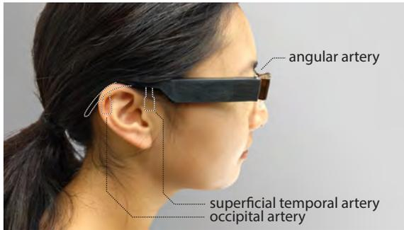
Fig. 15. During the screening session, we measured each participant's head dimensions to precisely fit the sensor on the location of their superficial temporal artery and occipital artery in the 3D printed case, respectively. The sensor on the participant's angular artery was fixed and embedded into the nose pad of the frame.
