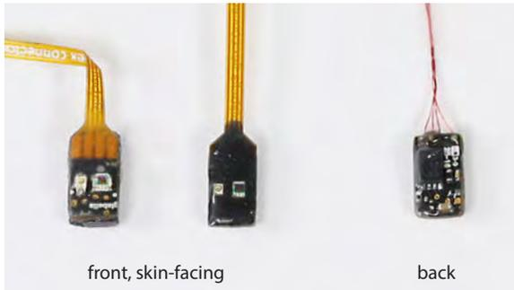
Fig. 6. Glabella’s sensor boards incorporate a photodiode, a corresponding and spectrum-matching green LED, and a small opamp circuit. The PSoC-integrated ADC on the main board digitizes all signals in synchrony. (Left) Custom FPC cables connect the two sensor boards in the frame to the main board. (Right) Thin magnet wires connect the sensor board that is embedded in the nose pad to the main board, routed along the frame for minimal visibility.
