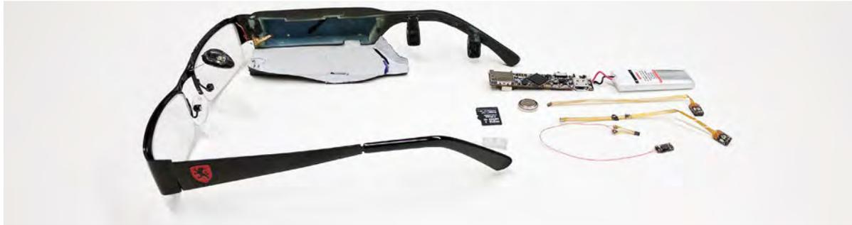
Fig. 4. Breakout view of a Glabella prototype. Two sensor boards are integrated into the glasses frame, one is seamlessly integrated into a nose pad. The main board includes storage and processing components and hides in the side frame alongside the battery.
