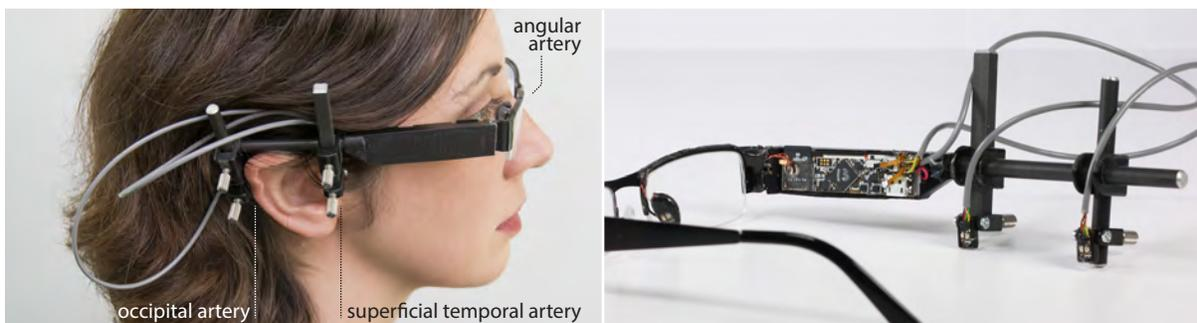
Fig. 14. Our adjustable lab prototype that recorded the pulse waves shown in Figure 13. While Glabella rigidly integrates the two sensor boards inside the frame at user-specific locations, this prototype features adjustable joints for translation, tilt, and rotation to fit a user’s head dimensions.
