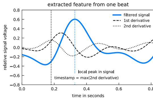
Fig. 11. Illustration of a single beat after applying a bandpass filter. We compute the feature timestamp from the local maximum of the 2<sup>nd</sup> derivative of each of the signals (dotted vertical line) just before the local peak of the signal (blue dotted vertical line).
