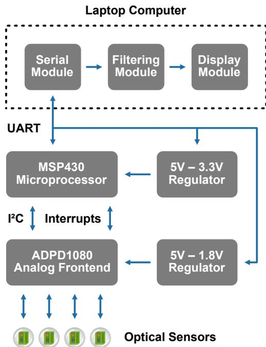
Fig. 2. Schematic of hardware and real time software modules.
