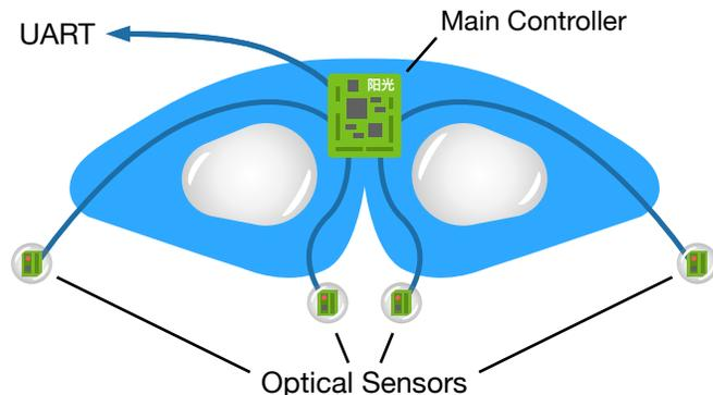
Fig. 1. Illustration of face mask with integrated optical sensing system
