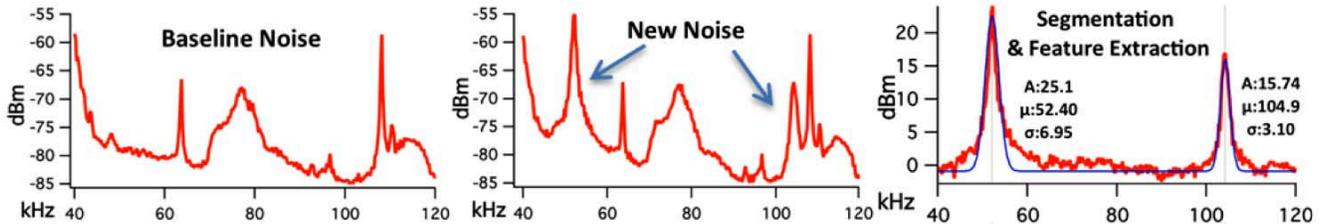
**Figure 6: (Left) Background noise observed on a particular power line. (Center) A new device is turned on, producing EMI that introduces new signals to the power line. (Right) After background subtraction the new signal features are extracted. The resulting Gaussian fit and its features amplitude (A), mean ( $\mu$ ) and variance ( $\sigma$ ) are also shown.**
