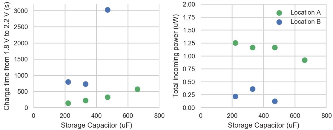
Fig. 8. Charge time and incoming power for different capacitors size
