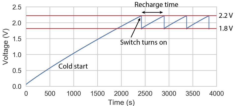
Fig. 5. When first installed, the harvester begins its cold start period. Once the storage capacitor reaches the trigger voltage of the high-side switch (2.21 V here), the switch activates and the device becomes active until the voltage drops to the lower cutoff voltage (1.8 V here). After that the recharge time of the device is significantly reduced.
