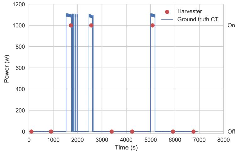
Fig. 10. Plot showing appliance state information (on/off) for a 1 kW hot plate measured using ApplianceTag along with ground truth data from collected using current transformer
