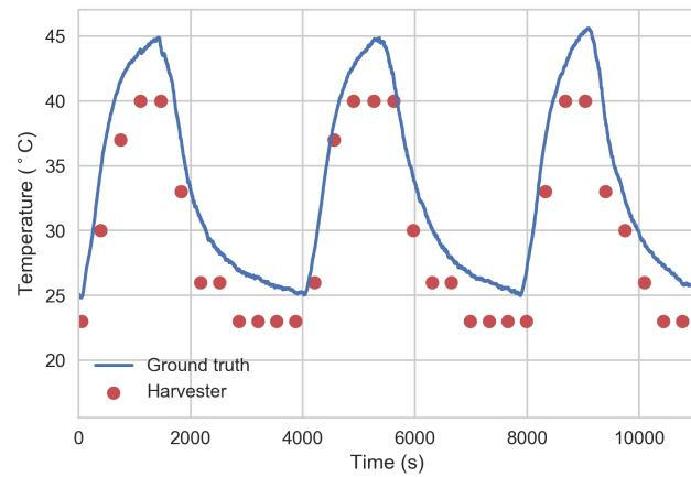
Fig. 12. Temperature variation logged using on-chip (TI CC1350) temperature sensor powered using capacitive harvester along with the ground truth data logged using high resolution temperature sensor (Texas Instruments HDC1000YPA)
