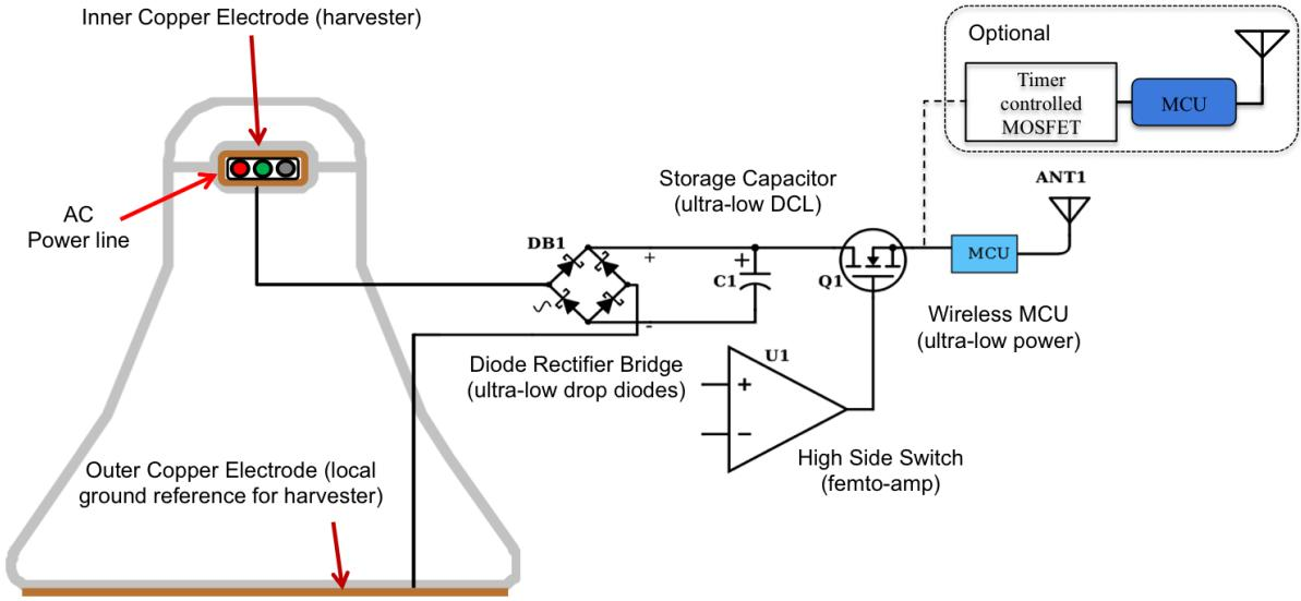
Fig. 4. The block diagram of our system, which consists of double-layer stacked capacitive electrodes, a diode rectifier bridge, a storage capacitor, a high side switch, and a wireless MCU for sensing applications. Optionally we also add a timer controlled MOSFET circuit to drive wireless MCU for continuous and event based sensing applications.
