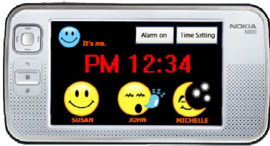
Figure 2. BuddyClock’s user interface on the Nokia N800. Users interact with BuddyClock using a touch screen display.
